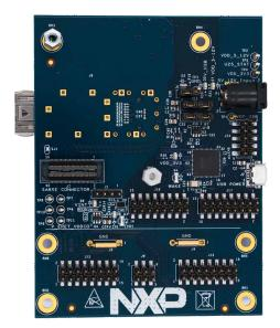
The TJA1120 evaluation kit enables the functional evaluation of the PHY and consists of the TJA11XX-EVB base board and TJA1120-SDBx adapter cards. The latter gets mounted via SABRE connector and carry the selected TJA1120 variant. To flexibly adapt to different application use cases, all configuration options can be selected via jumpers and all logic interfaces can be accessed via pin headers on the base board.
