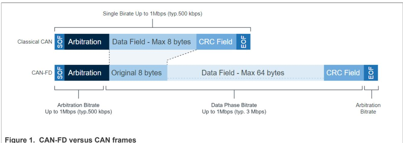
Figure 1. CAN-FD versus CAN frames
