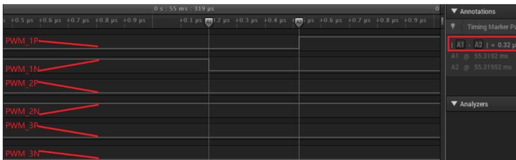
Figure 12. PWM waveform with dead time
