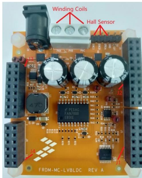
Figure 14. FRDM-MC-LVBLDC driver board
